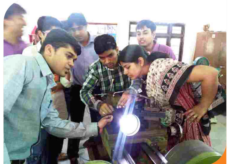
Speed measurement of lathe machine spindle using non-contact type (stroboscope)
