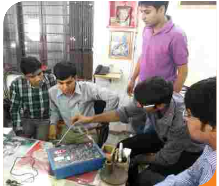
Temperature measurement of hot water using Resistance temperature detector
